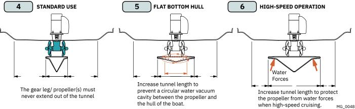
Some sail boats have a flat bottom and shallow draft in the bow section. This can make installing the thruster as far forward from the boats main pivot point difficult.
