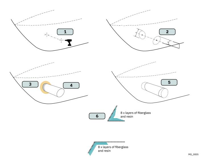
With tunnel installed and cast.
