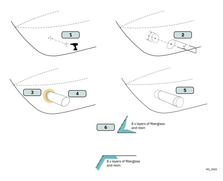
With tunnel installed and cast.
