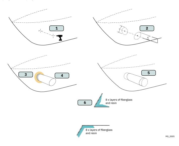
With tunnel installed and cast.
