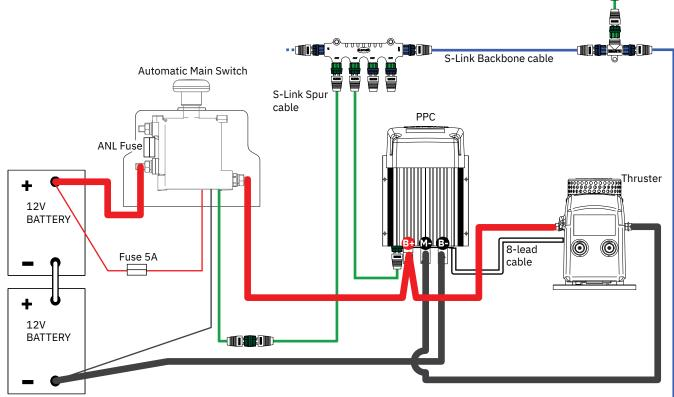
The top and bottom wiring setup is for a dual thruster system, For example bow and stern.
