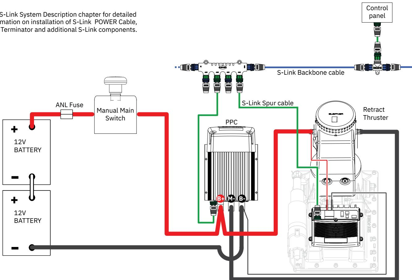
The top and bottom wiring diagram is for a dual thruster system, for example a bow and stern installation.
