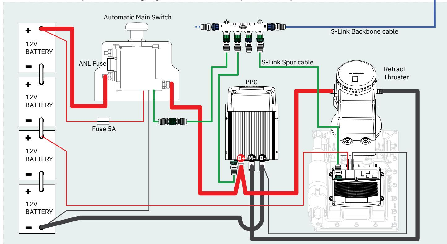
S-Link is a CAN-based control system used for communication between Sleipner products installed on a vessel. The system uses BACKBONE Cables as a common power and communication bus with separate SPUR Cables to each connected unit. Only one S-Link POWER cable shall be connected to the BACKBONE Cable. Units with low power consumption are powered directly from the S-Link bus.
