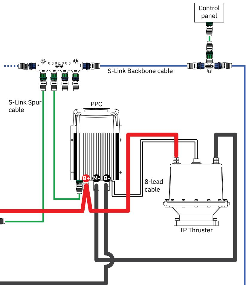
The top and bottom wiring setup is for a dual thruster system, For example bow and stern.
