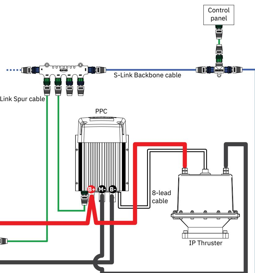
The top and bottom wiring setup is for a dual thruster system, For example bow and stern.
