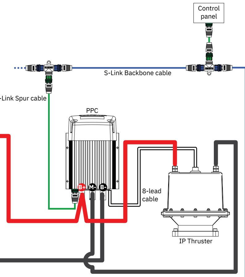
The top and bottom wiring setup is for a dual thruster system, For example bow and stern.
