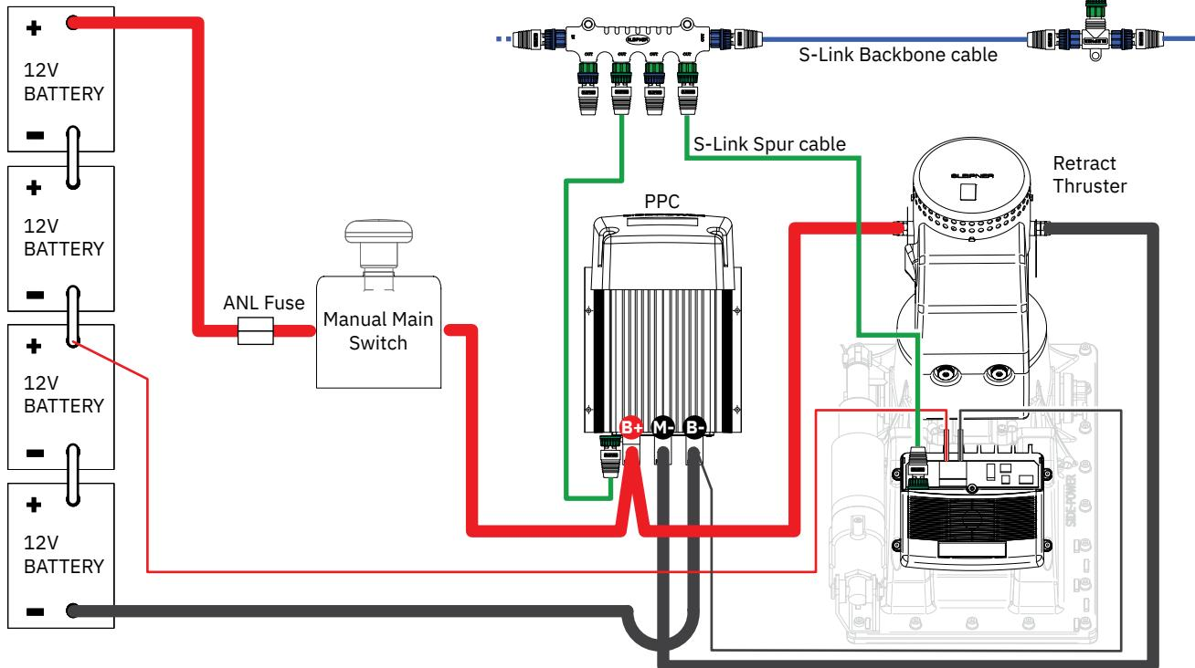
The top and bottom wiring diagram is for a dual thruster system, for example a bow and stern installation.
