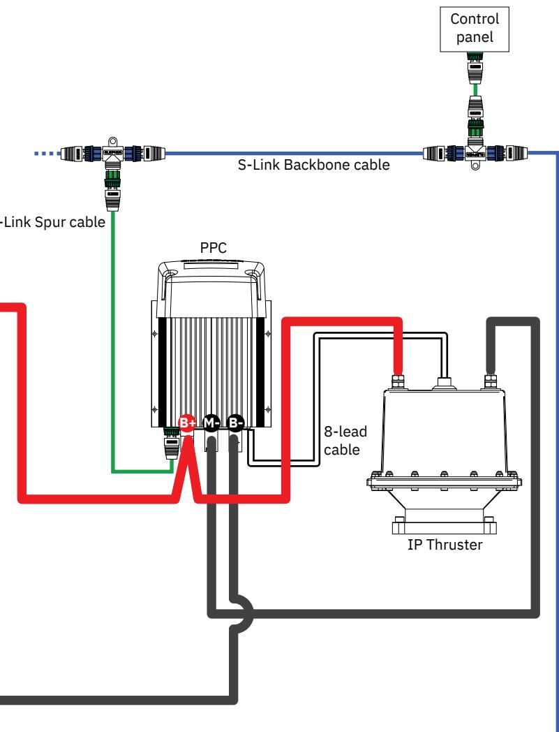
The top and bottom wiring setup is for a dual thruster system, For example bow and stern.
